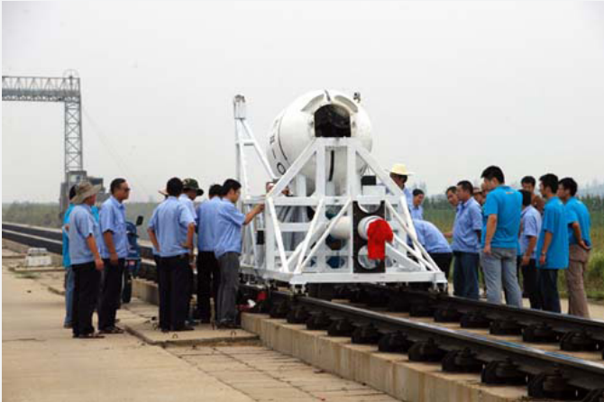
Rocket sled test of the Chang'e 5 recovery system (credit: Chinese Internet)
