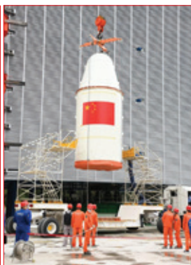
left: A CZ-2C takes off from XSLC with a new triplet of Yaogan satellites. Credit: Yu Ming/China Daily right: The CZ-2C payload fairing is lifted by a crane in September 2020. Credit: CASC
