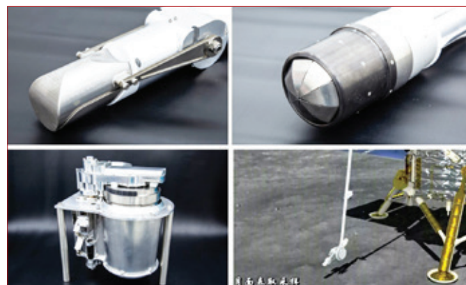
Hong Kong Polytechnic University's tools for Chang'e 5 include (clockwise from bottom left) a packaging and sealing system, a sampler for loose material, and another for sticky material – while Xinhua news agency's illustration (bottom right) shows how the samplers work with the probe's robotic arm. Photo: PolyU/Xinhua
