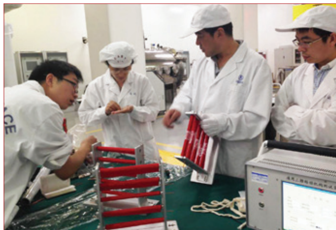
Engineers test the un-rolling mechanism at CAST. Credit: CAST/Wuhan Textile University
