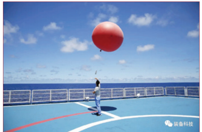
The beacon ball is released on board of YW-6 to check the tracking performance of the equipment. Credit: Xinhua
