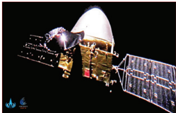
left: TW-1 as seen on its 1 st space selfie. The solar panels and the high-gain antenna are well recognisable. The silver-white section is the Mars entry module and heat shield, hosting the Mars rover. Credit: CNSA right: A map on the screen of BACC. It shows the Tianwen manoeuvre from 9 October. Credit: Xinhua/Cai Yang
