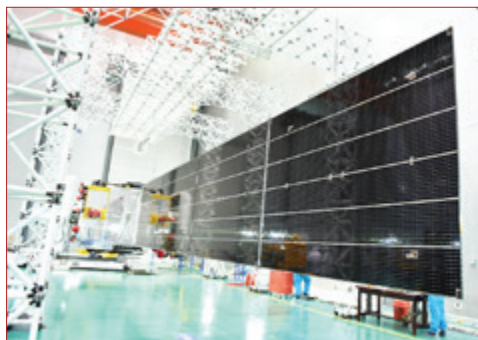
The APStar 6D satellite is equipped with a new generation solar panel system. Credit: CAST
