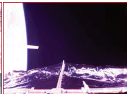
The external camera on Xiaoxiang 1-03 took this image after the in-orbit deployment of the de-orbit sail.
