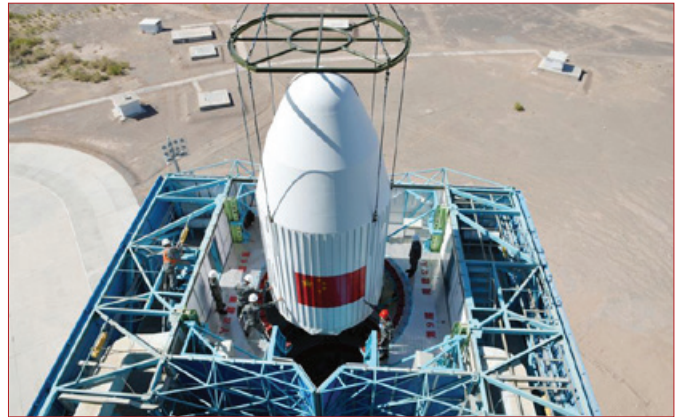
The CZ-2D carrier rocket is assembled in the launch tower at the Jiuquan Satellite Launch Centre. Credit: Wu Jiadong/Ti Gong
