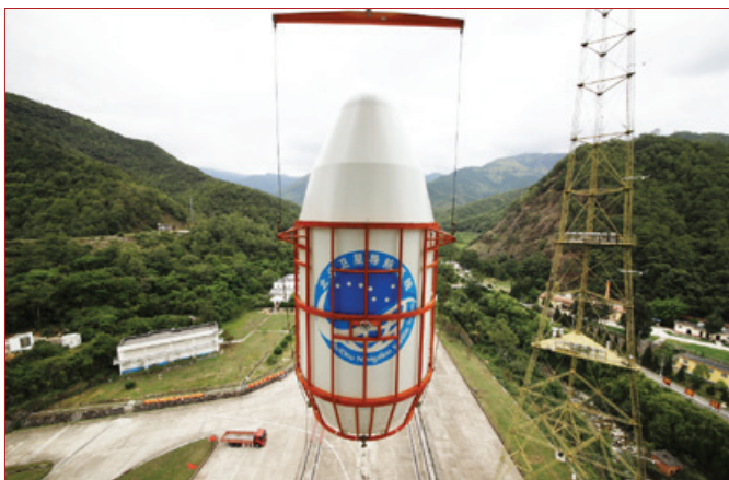
The fairing is lifted to the CZ-3B carrier rocket at the Xichang Satellite Launch Centre in Southwest China's Sichuan province. Credit: CALT/Ning Hong, CGTN
