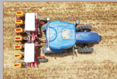
An unmanned tractor equipped with a Beidou navigation system sows a new crop in the village of Anzhong in Dengzhou, Henan province, on 26 May. Credit: Feng Dapeng/Xinhua
