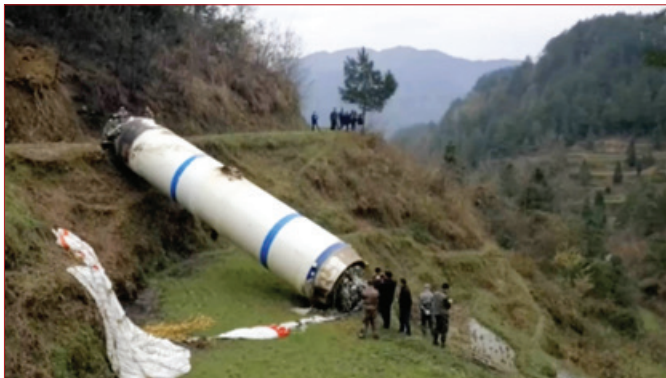
CZ-3B booster after landing by parachute. Credit: CCTV
