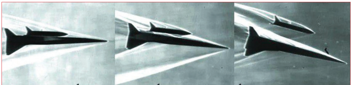
Hypersonic Space Plan - After the launch, the smaller vessel will separate to deliver its payload into space. Credit: Handout/SCMP
