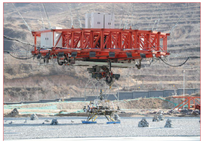
Mars landing simulator where the process of hovering, avoiding obstacles and descending to land on Mars was tested on 14 November 2019. Credit: Xinhua/Jin Liwang
