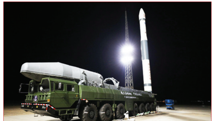
The road-mobile transport vehicle and launch pad for the Kuaizhou 1A rocket is being prepared. Credit: Expace/People's Daily
