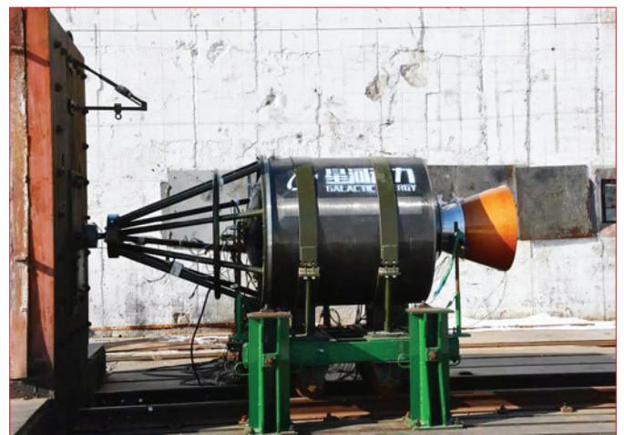
Galactic Energy's 3 rd stage in test stand. Credit: Galactic Energy
