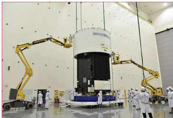
left: Shijian 20, a technology demonstration satellite developed by the China Academy of Space Technology in Beijing, gets encapsulated for the launch with the Long March 5 carrier rocket at Wenchang Space Launch Centre in Hainan province. Credit: China Daily/Zhuang Qianqian middle: Fisheye view of the CZ-5 in the assembly building. right: Launch of the CZ-5 with the SJ-20 satellite on board from Wenchang Space Launch Centre on Hainan Island. Credit: GuoWenbin/Xinhua
