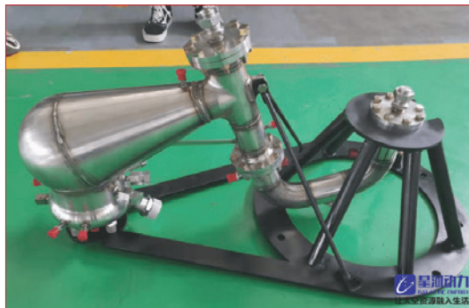
Galactic Energy's Multiple Counterflow Vortex Unique Configuration Gas Generator – the key component for the Pallas 1 rocket engine. Credit: Galactic Energy
