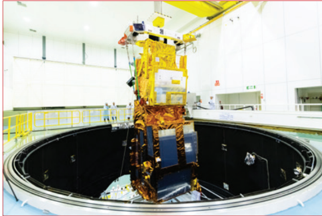
During the visit to ESTEC, the MetOp-2 nd generation satellite was visible through the open hatch of the Large Space Simulator, the largest vacuum chamber in Europe. On this archive photo the MetOp's structural and thermal model is being lowered into the Space Simulator, ahead of thermal vacuum testing during summer 2019. ESTEC's test facility also houses Europe's loudest sound system, used to expose satellites to simulated launch noise. Likewise, Europe's most powerful shaker table is hosted at ESTEC. Credit: ESA-SJM Photography
