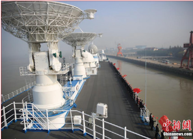
A close-up of the antenna facilities on Yuanwang 7 while departing from its home port on 26 November 2018 to carry out maritime space monitoring and communication missions. credit: Chinanews.com
