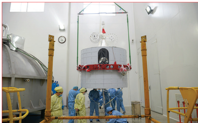
The Fengyun-2H weather satellite during space environment testing. credit: CASC
