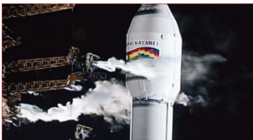
The TKSat is mounted in a protective cover, sitting on top of its launcher, the CZ-3B. credit: Xinhua
