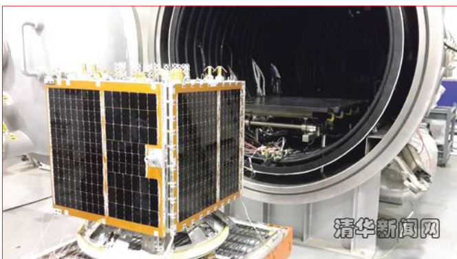
The Xinwei SCES satellite in front of the vacuum test chamber. Credit: Xinwei/internet
