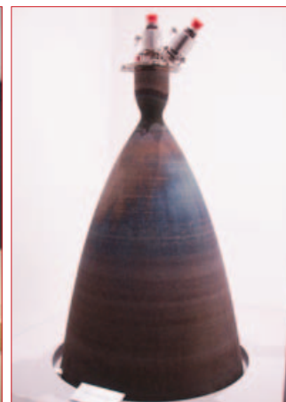
The liquid-fuelled, 2,500 N twin-engine developed by the 6 th Academy of China Aerospace Science and Technology Corporation (CASC) is used for the Shenzhou space craft in case of emergency escape, orbital and return manoeuvring. credit: GoTaikonauts!
